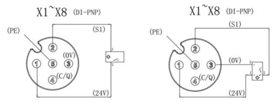
2. PNP type output signal, that is, the jack is connected to the actuator.
