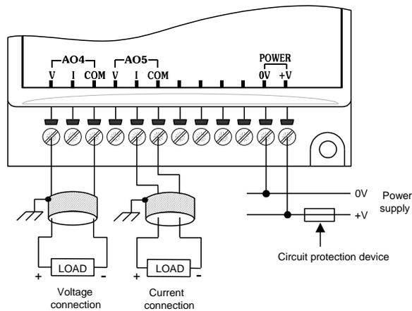
**Wiring the Analog Outputs' Power Supply**
