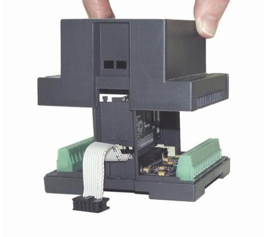
4. The jumpers are shown at right. Change the jumper settings as required, in accordance with the tables shown on the next page.
