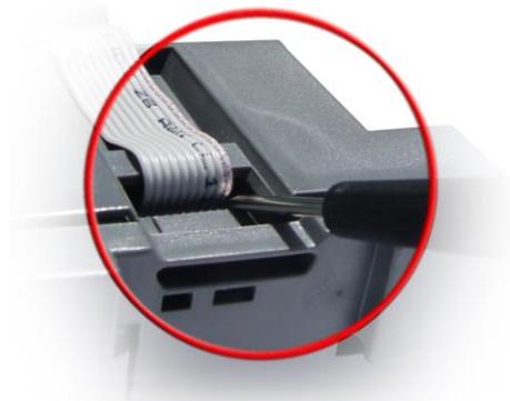
3. Gently remove the top of the device as shown.
