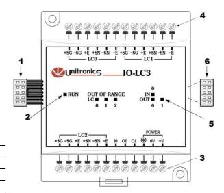
**Note:** The single Loadcell input offered by IO-LC1 is marked LC and is located where the input LC2 is shown above.
