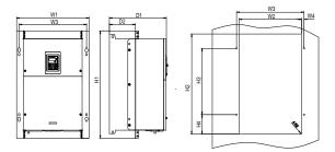
Flange mounting of 3PH 400V 90-110kW inverters (dimension unit: mm)
