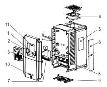
Figure 2-4 Product structure (Three phase 400V, ≥4kW)
