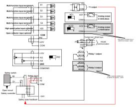
Figure 3-9 Wiring of control circuit
