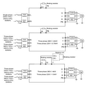
Figure 3-3 Connection diagram of main circuit
