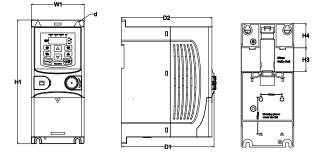
Rail mounting of inverters of 1PH 220V/3PH 380V (<2.2kW) and 3PH 220V (<0.75kW) (dimension unit: mm)
