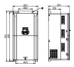
Wall mounting of 3PH 400V 45-75kW inverters
